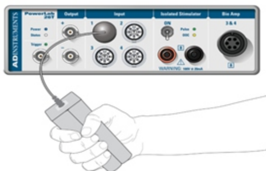
Fig. 2: PowerLab Hardware with Handgrip dynamometer and its Digital graph for Fatigue time*.
